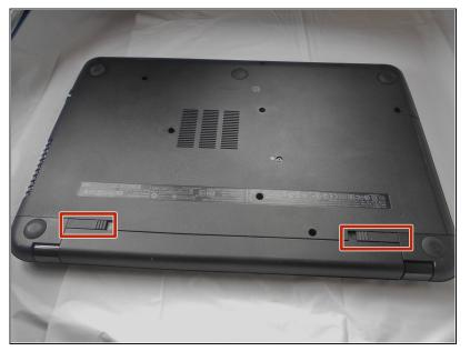
• There are two battery release switches circled.
