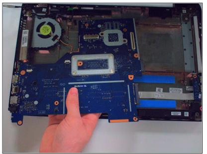
• After removing all the wires, pull the motherboard out.
