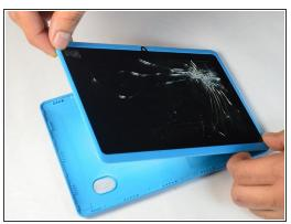
Place your Plastic Opening Tool between the screen and the case. Slowly move it around the casing while prying in a downward motion to undo the hinges holding the two together and separate the two parts.
