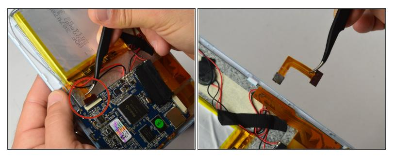
Using a pair of tweezers, gently grasp the flex cable and pull it out while using your other hand to keep the camera in place. Once removed, your camera is now free to set aside.
