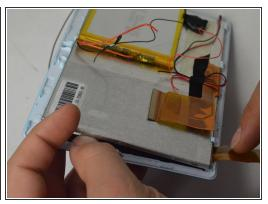
Using your Plastic Opening Tool, pry between the plastic casing and the screen to free it. Once free, you may begin separating the screen from the casing.
