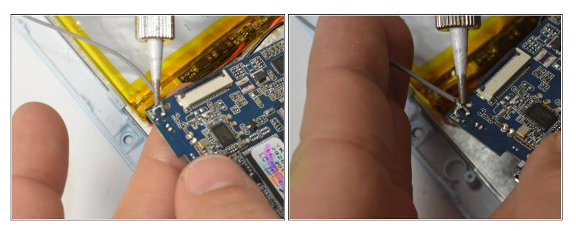
Using your soldering Iron, desolder the grounding cable on the motherboard.
