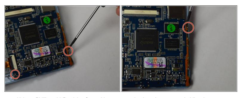
Using a Phillips #00 Precision Screwdriver, remove the three 3mm screws holding the motherboard.
