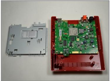
• Lift out the metal plate and set it aside.
