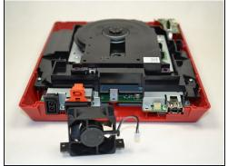
Using your fingers, gently pull the top of the pin connector straight up to detach the fan from the console.
