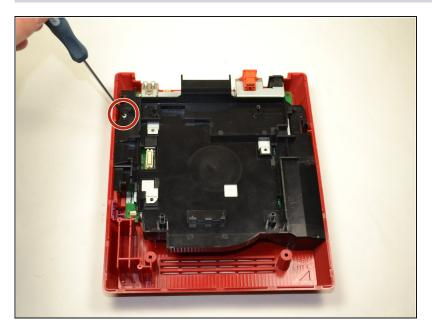
Using a Phillips #0 Screwdriver, unscrew the 6 mm screw at the top of the black tray.
