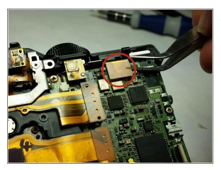
Once both the front and rear covers are removed, disconnect this ribbon cable by flipping it up and disconnecting it.
