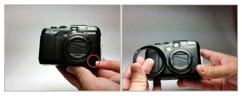
Push the button on the bottom right of the camera and then remove the plastic surrounding the lens.
