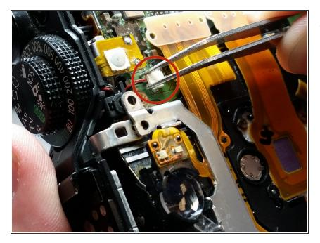
Disconnect this cable from the motherboard by sliding it in the direction of the cable (toward the top of the camera).
