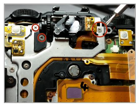
• Remove these three screws from the rear side of the camera.
