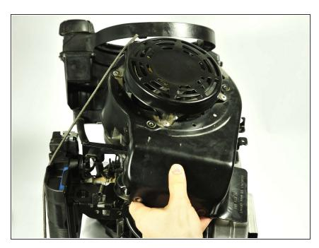
Remove the engine shield and flip it over.
