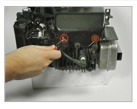
Use a socket wrench with a 3/8" socket to remove the two 20mm screws on the front of the engine shield.
