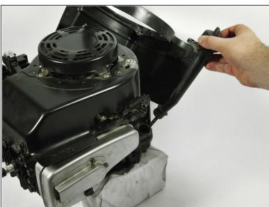
Remove the oil funnel from the rest of the engine. It should pull away easily and come off completely.
