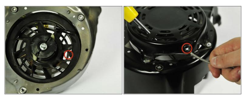
• Line up the hole on the outside of the engine shield with the hole on the inside, then slip the new pull cord through and tie a knot.
