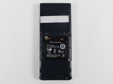
Remove the back plate using the spudger or by hand.
