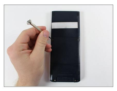
Replace the back plate and the 2 screws.
