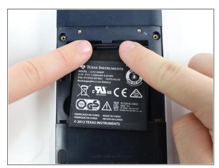
Position the new battery and tuck the wire under the tab.
