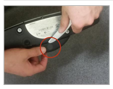
Use a plastic scraper to remove the rubber gasket from the bottom of speaker system and set it aside.
