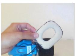
• Remove the cushion from the headphones by carefully pushing the edges out from the sides of the ear piece.
