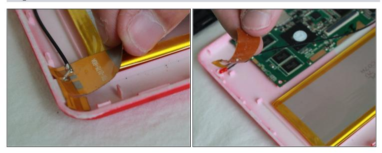
• Peel off the tape that is attaching the wifi antenna to the case.
