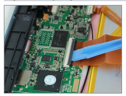
• With the plastic opening tool, lift the black latch up.
