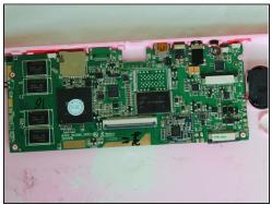
• Using the screwdriver, remove the four 4mm by 1.5mm screws that are attaching the motherboard to the case.
