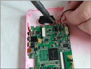
• Using the soldering iron, heat up the solder that is attaching the battery to the motheboard.
