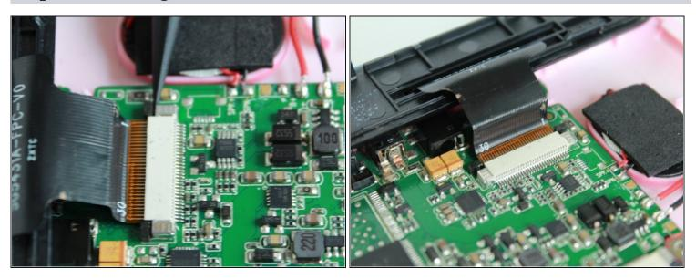
• Use the tip of the spudger to release the latches on the motherboard.
