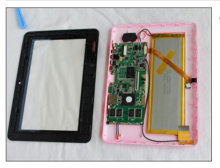
Remove the cable from the motherboard.
