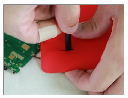
Insert the spudger into the speaker slot on the back of the case.
