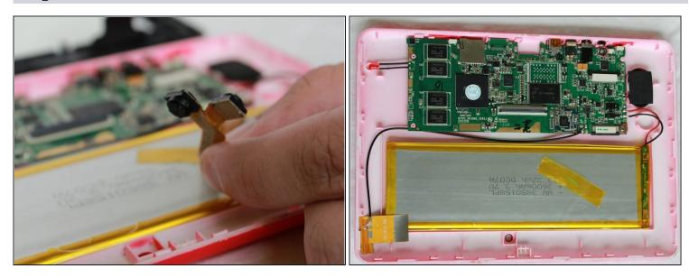
• Remove the camera from the device.
