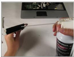
Remove dust trapped in the heat sink vent with compressed air and/or a small brush.
