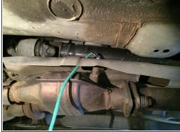
Unplug the rear oxygen sensor connector and carefully route the wires through the Exhaust Front Cover so they are no longer passing through it.
