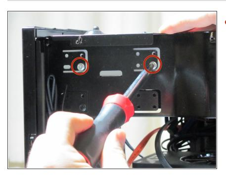
Locate and unscrew the screws holding the CD drive to the case.
