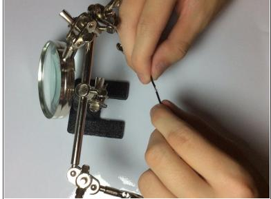
Using both stripped wire ends, wrap and tie both of the ends together.
