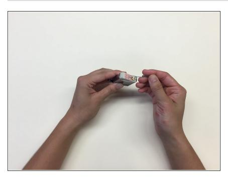
Unravel the paperclip. Lodge one end of the paper clip into the tiny hole and lift up the felt backing.
