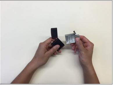
Open the lid of the Zippo and extract the insert – firmly grip either side of the flint wheel with 2 fingers. Hold the bottom of the Zippo lighter with your other hand and pull up on the metal to free the insert of the lighter from its case.
