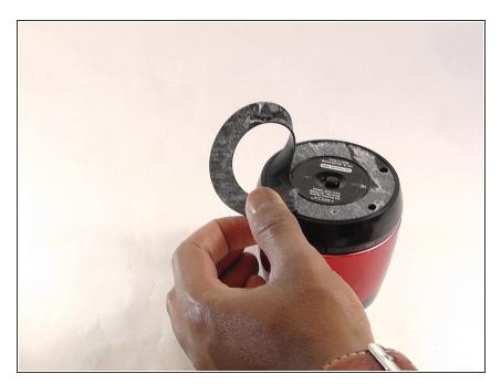
Carefully replace the old rubber with the new one, being mindful to line the cover up correctly with the outside edge of the device as well as the inner cover.
