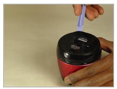
Pry off the rubber cover at the bottom of the speaker by using the plastic opening tool.
