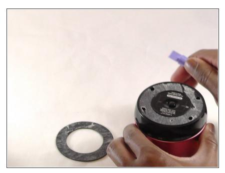
After completely removing the rubber cover, find a new cover and prepare both it and the device for attachment.
