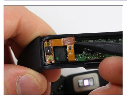
Using the spudger or the plastic opening tool, gently lift the sensor ribbon.
