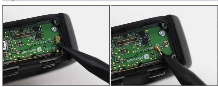
• Using the spudger or the <u>tweezers</u>, gently detach the golden connector from the motherboard.
