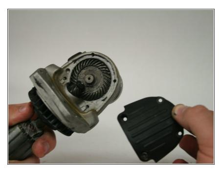
Remove the gear case cover from the gear case.
