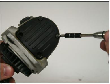
Using the T-15 screwdriver, remove the four torx screws.
