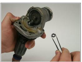
Using a 10-mm wrench, remove the hex nut by rotating counter-clockwise.
