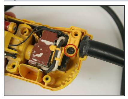
Remove the single 20-mm torx screw holding the rear panel in place.
