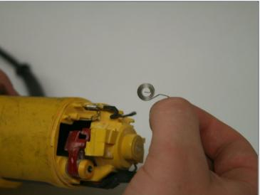
• Use the edge of the spudger to slide the spring off its post.
