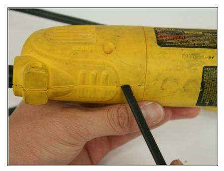
• Use the edge of the spudger to loosen and remove the back panel.
