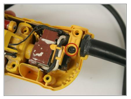
Remove the single 20-mm torx screw holding the rear panel in place.
