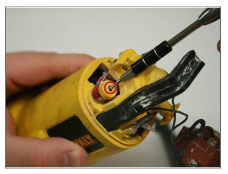
• Using the T-6 screwdriver, unscrew torx screw holding the arm in place.
