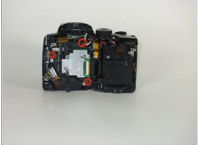
• Use a PH00 screwdriver to remove the three labeled 3mm screws.
