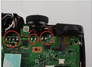
Desolder the labeled soldering points.
