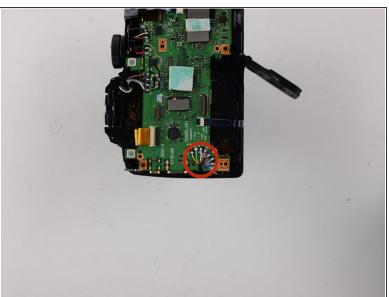
Desolder the labeled soldering points.
