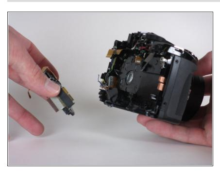
Remove the black plastic holding the image sensor from the camera. You now have access to the front casing of the camera.
