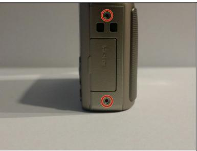
• Using a small screwdriver, remove the four 3.4mm screws from the right and left sides of your Panasonic Lumix Camera.
