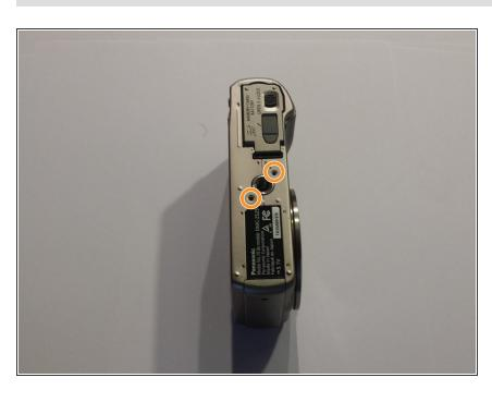
Using a small screwdriver, remove the two 2.6mm screws located next to the battery, on the outer casing.
