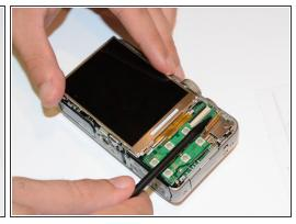
• Using the spudger, pull upward on the screen cable to release it.
