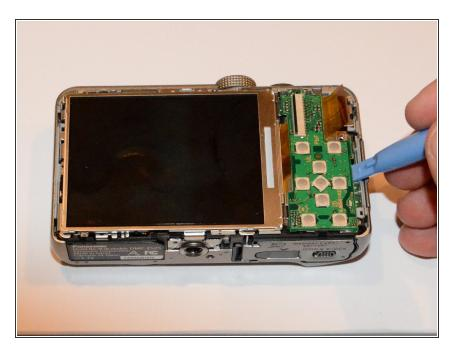
Using the plastic opening tool, lift the button board until it clicks.
