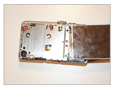
Using a small screwdriver, remove the two 4.2mm screws located on the corner of the inner cover, under the screen.
