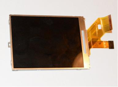
Remove the screen using the iFixit opening tool.
