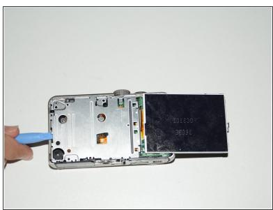
Open the two 4.20 mm screws to remove the inner cover located beneath the screen.
