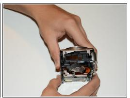
Remove the side cover using the iFixit opening tool.
