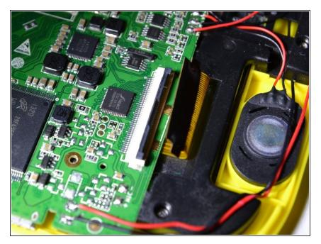
Pull the three ribbon cables out so that they are no longer connected to the logic board.
