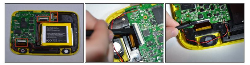
Use the flat end of the spudger to lift the black panels covering the three ribbon cables connected to the logic board.
