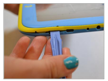
Use the plastic opening tool to unclip the plastic front from the plastic back. Use the MicroSD slot to initially start the unclipping.
