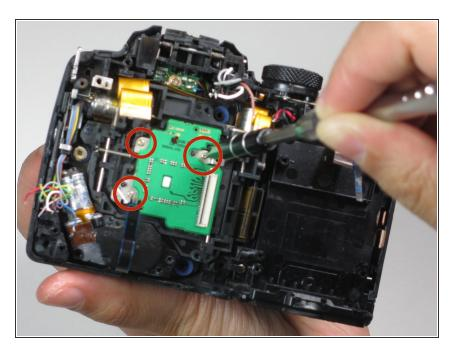
Use a PH00 screwdriver to remove the three 3mm screws holding the image sensor down.
