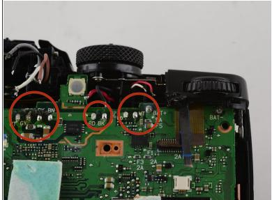
Desolder the labeled soldering points.
