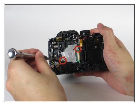
Use a PH00 screwdriver to remove the two 2mm metal screws from the image sensor cover.
