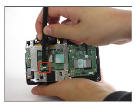
Use a spudger to flip up the cable lock in order to release the ribbon.
