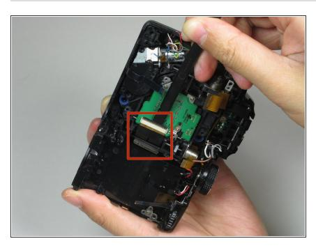
Use a spudger to unlock the connector ribbon.
