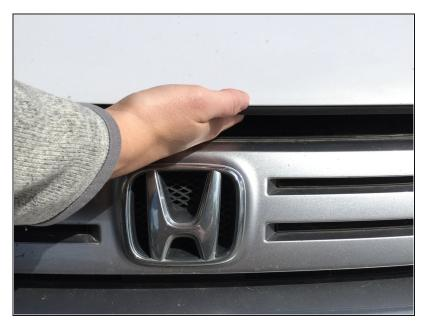
Open the hood by reaching under the hood (in the front and center) and pulling the lever.
