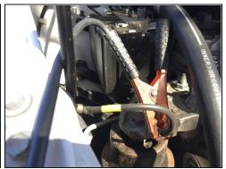
• Attach the other BLACK lead to the grounding strap located here:
