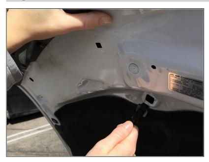
Lock open the hood by grabbing the rod and inserting it into the hole on the under side of the hood.
