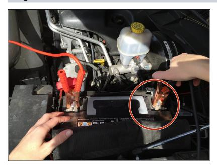
Attach the BLACK lead to the secondary car's battery where the negative terminal is.
