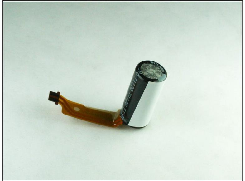
**⚠ Caution:** Touching the capacitor wires may cause serious injury. Use a [capacitor discharge probe](#) to safely rid the capacitors of dangerous charges.
