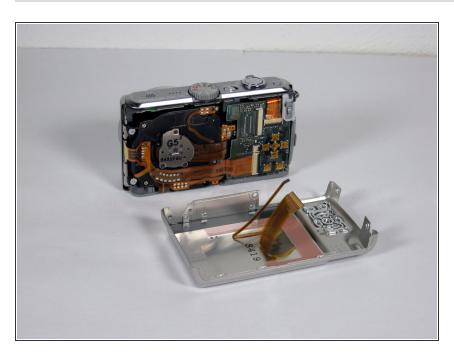
Remove the back casing from the camera.
