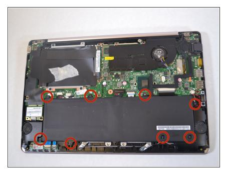
Remove the eight 4.7mm Philips #00 screws holding the battery in place.
