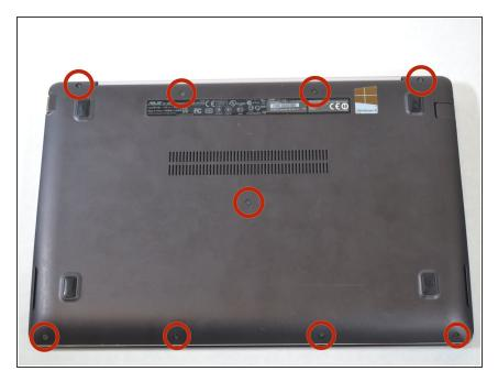
Remove the nine Philips #00 screws holding the back panel in place (four 5.6mm, four 7.7mm, and one 9.2mm).
