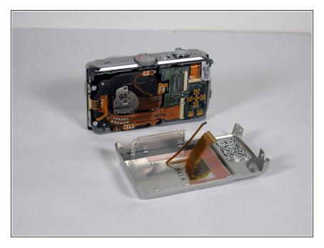
• Remove the back casing from the camera.
