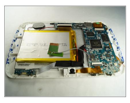
Locate the battery. Generally located in the middle of the device.
