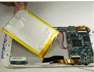
Carefully pry off the battery from the display screen. This will be slight difficult since the battery is held onto the back of the display by adhesive.
