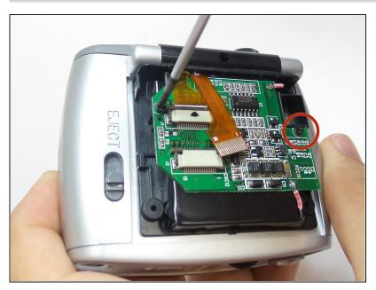
Remove the two black screws from the circuit board.
