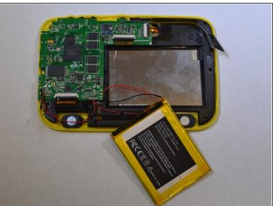
The battery is glued onto the black plastic. Use the plastic opening tool to pry the battery from the black plastic.
