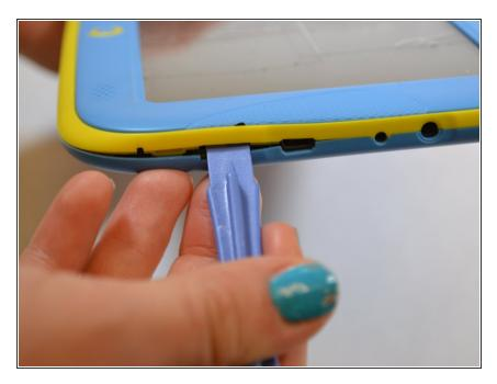
Use the plastic opening tool to unclip the plastic front from the plastic back. Use the MicroSD slot to initially start the unclipping.
