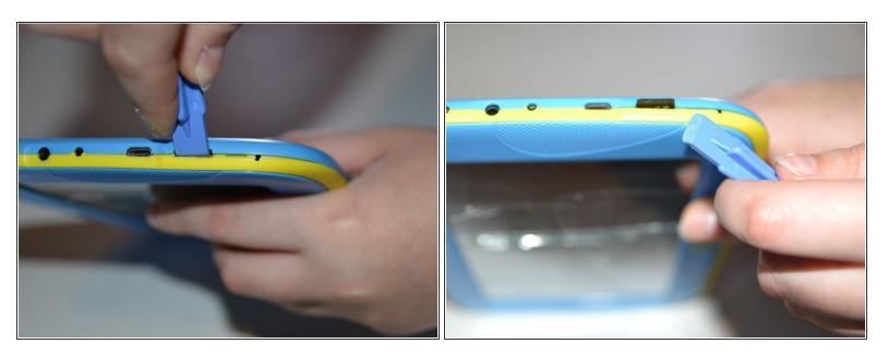
Use the plastic opening tool help push out the microSD card from the microSD slot.
