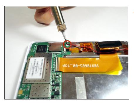
Desolder the two leads of the speaker wire that are connected to the motherboard.
