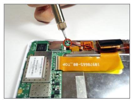
Desolder the two leads of the speaker wire that are connected to the motherboard.
