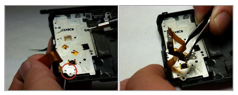
• After the screws are removed, pull the metal bracket out of the camera.
