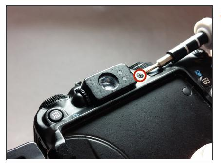
Remove the screw to the right of the view finder on the rear of the camera.
