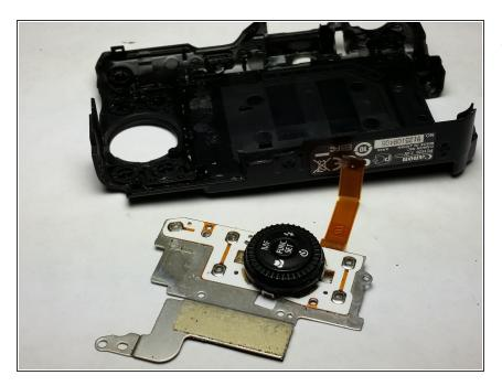
• Remove the dial from the case completely.
