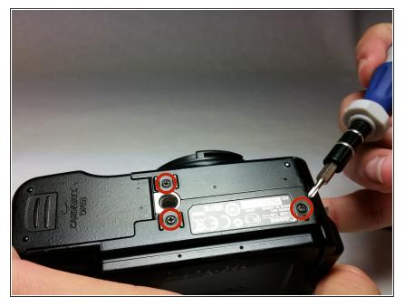
Remove the three screws on the bottom of the camera using the 00 sized phillips head screw driver.
