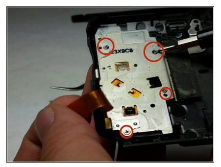
Remove the four screws that are now accessible with the removal of the plastic covering them.
