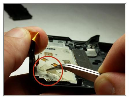
• Remove the plastic covering of the left side of the rear case interior.
