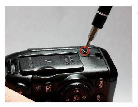
Remove the screw on the right side of the camera.
