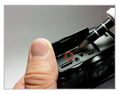
Open up the HDMI port on the right side of the camera. Then remove the screw in the HDMI port.
