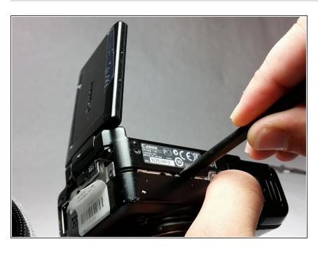
Use the spudger to crack open the case.
