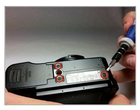
Remove the three screws on the bottom of the camera using the 00 sized phillips head screw driver.
