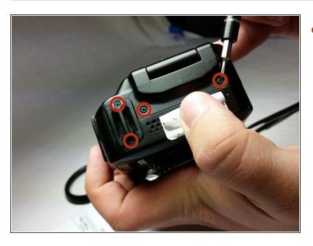
Remove the four screws on the left side of the camera.
