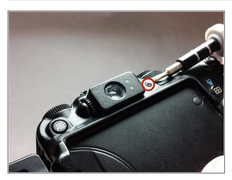
Remove the screw to the right of the view finder on the rear of the camera.
