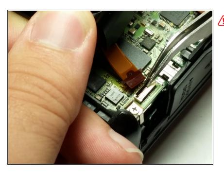
The rear case is still attached to the camera with a ribbon cable. The socket has a flip up lid that must be flipped up before the cable can be removed. Use the tweezers to flip the cable attachment up.
