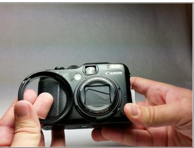
Push the button on the bottom right of the camera and then remove the plastic surrounding the lens.
