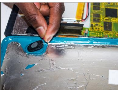
Carefully peel the tape holding down the wires connected to the speaker.
