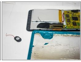
Remove the speakers by using your hand to entirely disconnect the back cover.
