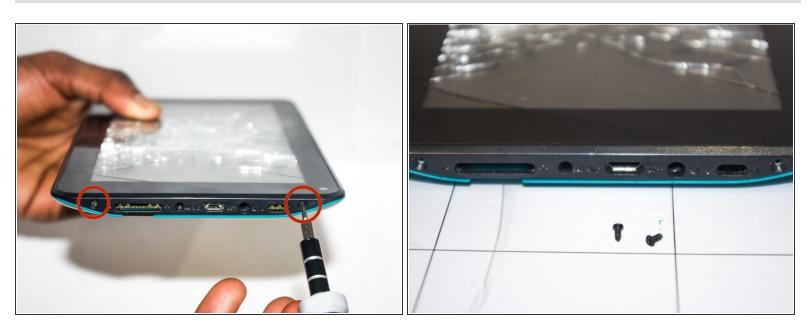
Remove the two 1.2 mm Phillips #0 screws found at the side by the power button.
