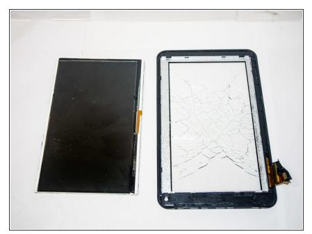
After pulling out the screen, what you have left is the digitizer, which is what allows the tablet to recognize your touch.
