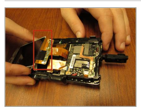
Carefully unclip the screen from its circuit ribbon.
