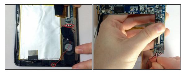
• Once the screws are removed, you should fully desolder the speaker wires that are attached to the motherboard. Instructions on how to desolder these wires are here on ifixit: <u>How To Solder and Desolder Connections</u>
