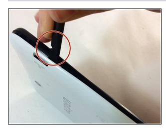
• Use the plastic opening tool or black spudger tool to lift the back panel off the tablet.
