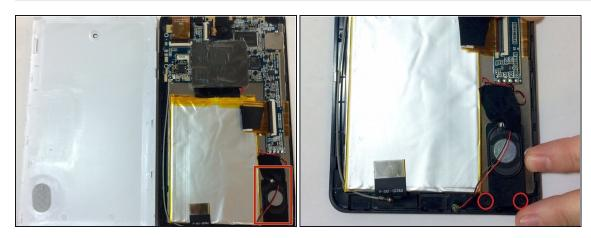
• The speaker will be attached by 2 screws with 3.75mm and 3.81mm at the bottom of the plastic holding the speaker in. These 2 screws will need to be removed in order to replace the speaker with a pentalobe screwdriver.
