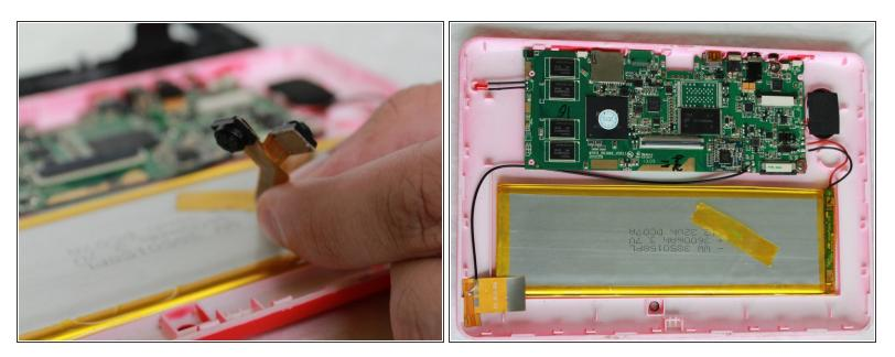
• Remove the camera from the device.
