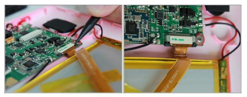
• Use the tip of the spudger to release the latches on the motherboard.
