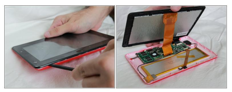
• Slide the spudger along the perimeter of the device to fully separate the two pieces.
