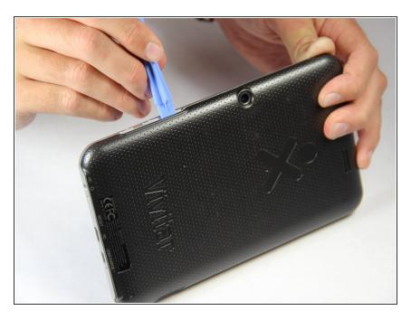
With the plastic opening tools, pry open the back cover.
