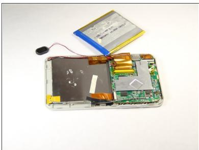
Carefully remove the battery from the tablet.
