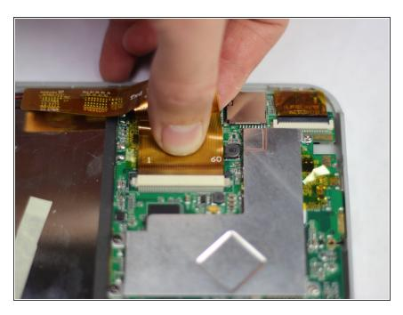
Disconnect the large golden ribbon cable that is connected to the digitizer. Firmly grab the cable close
