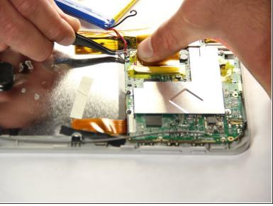
With the tweezers, firmly grab the wire at the base and pull to disconnect the battery from the motherboard.
