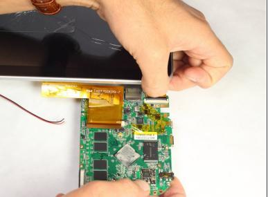
Gently pick up and turn over the motherboard. While turned over, disconnect the last ribbon cable that connects to screen.
