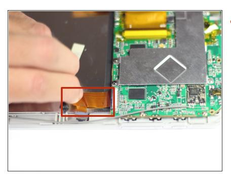
Carefully disconnect the ribbon cables from the motherboard.
