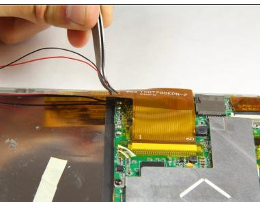
Using the tweezers, firmly grab wires and pull to disconnect them from the motherboard.
