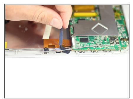
Peel off black tape that is holding the camera in place.
