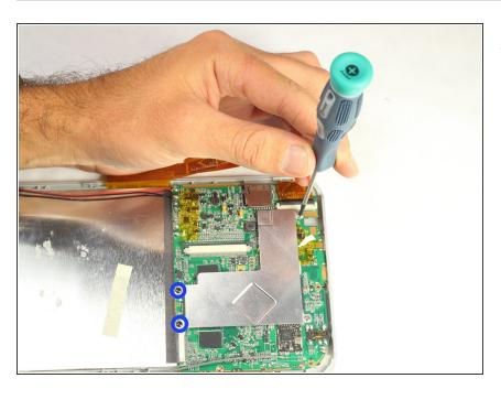
Remove two 2mm PH00 black screws from the motherboard.
