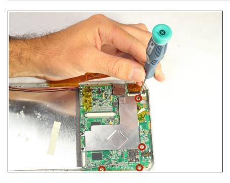
Remove four 4mm PH00 silver screws from the motherboard.
