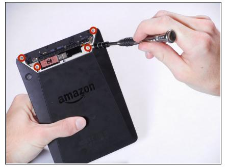
• Use an aluminum driver attached with a Phillips head size #00 to remove the four 3mm screws shown in the picture. For reassembly, note that the top two and bottom two screws are different sizes.
