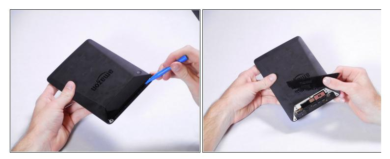
• Insert a plastic opening tool between the plastic panel shown on the device.
