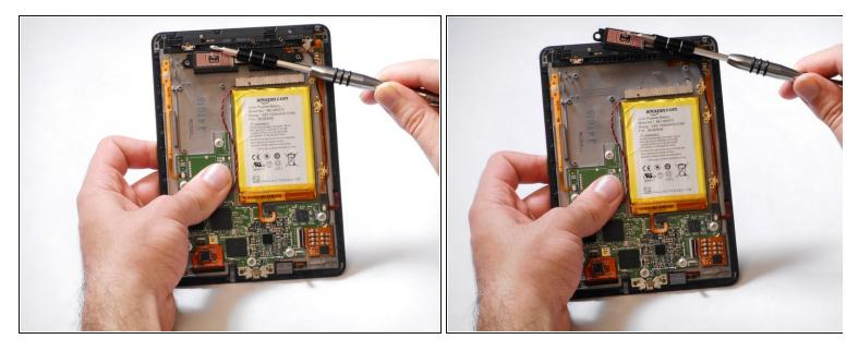
• Remove the magnetic component with the magnetic head of the aluminum driver.
