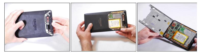
• Once the screws are removed, the back panel can slide off the device.
