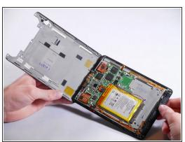
Once the screws are removed, the back panel can slide off the device.
