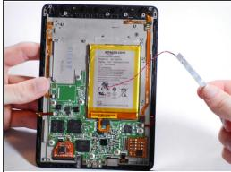
Gently peel the vibrator off of the device.
