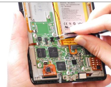
Use tweezers to pinch in the sides of the vibrator cable and slide it out of its housing.
