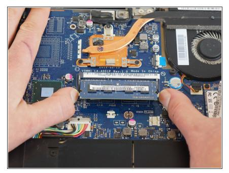
Push the retaining clips away from the RAM module, allowing the spring loaded hinge to pop up.
