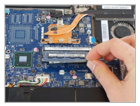
• Carefully pull the RAM module away from the motherboard.
