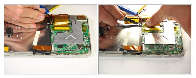
• With the tweezers, firmly grab the wire at the base and pull to disconnect the battery from the motherboard.
