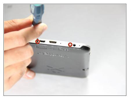
• Remove the two 3mm Phillips #00 screws on the bottom of the tablet.
