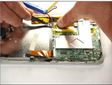
• With the <u>tweezers</u>, firmly grab the wire at the base and pull to disconnect the battery from the motherboard.
