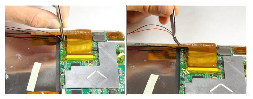
• Using the tweezers, firmly grab wires and pull to disconnect them from the motherboard.
