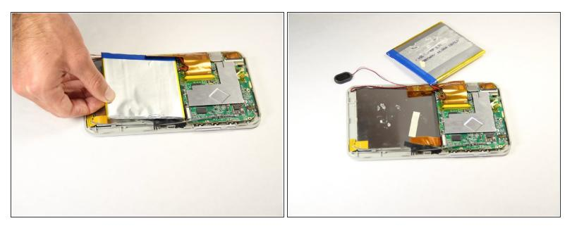
• Carefully remove the battery from the tablet.
