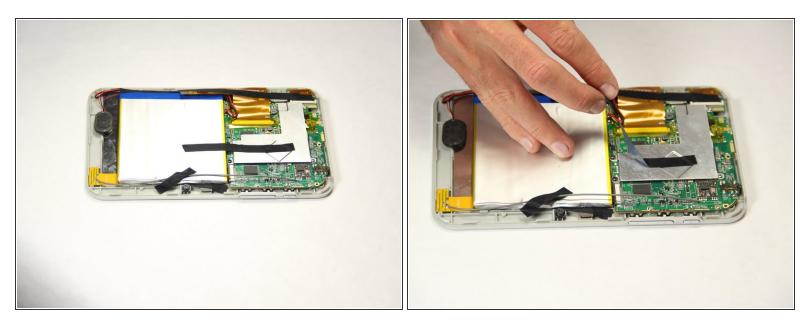
• Peel off the black pieces of tape from the internal components.
