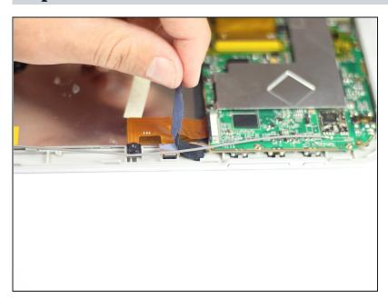
Peel off black tape that is holding the camera in place.
