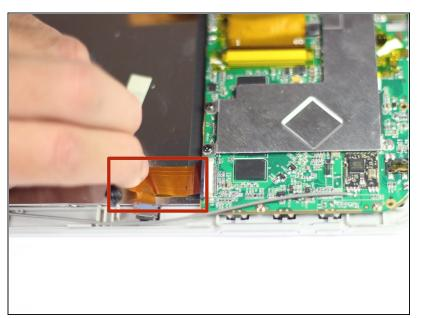
• Carefully disconnect the ribbon cables from the motherboard.
