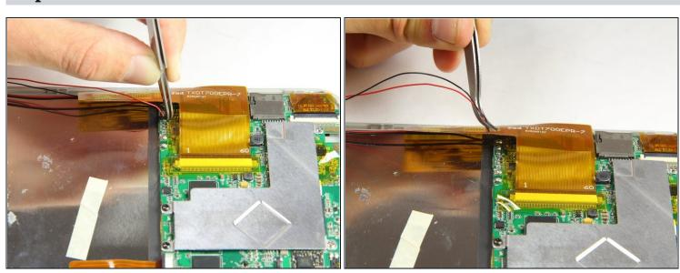
• Using the <u>tweezers</u>, firmly grab wires and pull to disconnect them from the motherboard.
