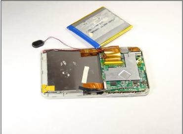
• Carefully remove the battery from the tablet.
