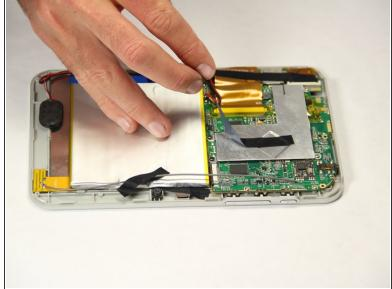
Peel off the black pieces of tape from the internal components.
