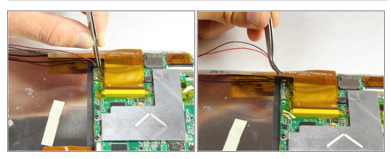
With tweezers, firmly grab the wire at the base and pull to disconnect the speaker from the motherboard.
