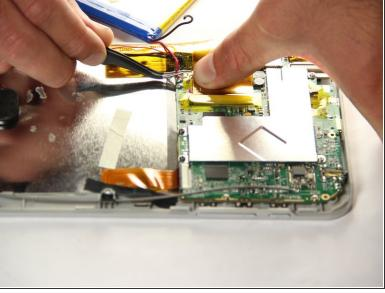
With the tweezers, firmly grab the wire at the base and pull to disconnect the battery from the motherboard.
