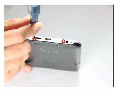
Remove the two 3mm Phillips #00 screws on the bottom of the tablet.
