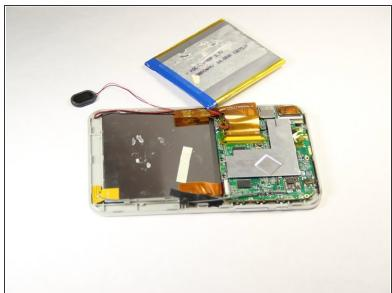
Carefully remove the battery from the tablet.
