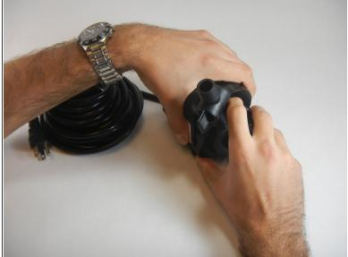
• Firmly hold the pump block with one hand and the impeller housing with the other hand. Rotate impeller housing counterclockwise until it is released.
