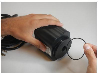
With one finger from the hand that is holding the pump, push the lifted portion of the ring forward until it is completely detached from the pump.
